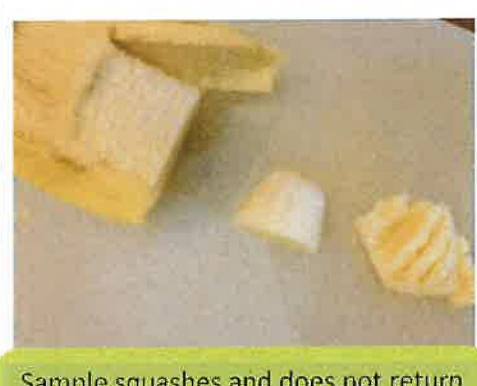
Sample squashes and does not return to its original shape when pressure is released
